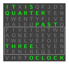
Figure 1: Example word clock displaying the time 3:15. Note that for efficiency reasons, words are allowed to overlap, e.g. FIVE and EIGHT.
